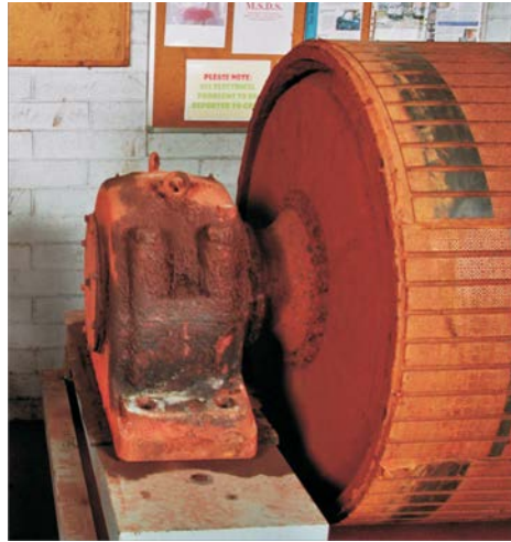
Above: An unprotected pulley housing - and a similar pulley after refurbishment. Below: With the Enviropeel removed from a pulley housing after use, it is clear how good the performance of the Enviropeel is. The roller in the background shows clear evidence of corrosion whereas the protected pulley is as good as new.
