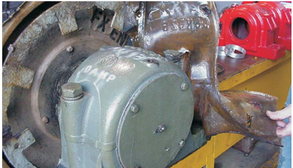
Above: An unprotected pulley housing - and a similar pulley after refurbishment. Below: With the Enviropeel removed from a pulley housing after use, it is clear how good the performance of the Enviropeel is. The roller in the background shows clear evidence of corrosion whereas the protected pulley is as good as new.
