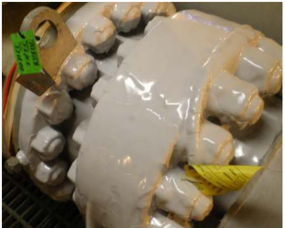
Application builds coats in succession, working from underneath, around the sides and finally above with two coats to provide maximum protection. The underside is the most difficult area to finish aesthetically but trimming between and after each coat ensures full protection. All trimmings and drips/spills are collected and recycled.
